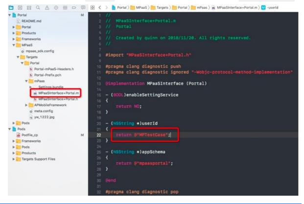
2. During user switching, that is, when the value configured in the userId function of MPaasInterface changes, call the following function:
